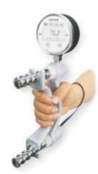
BMI-1173 **DIGITAL HAND DYNAMOMETER** (WITH SOFTWARE)
